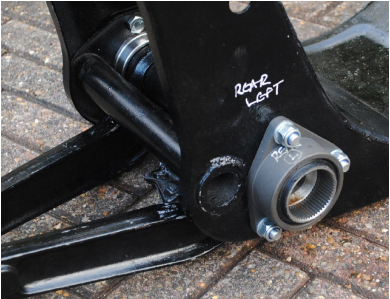
Fig 9 Silent blocs fitted to cradle
