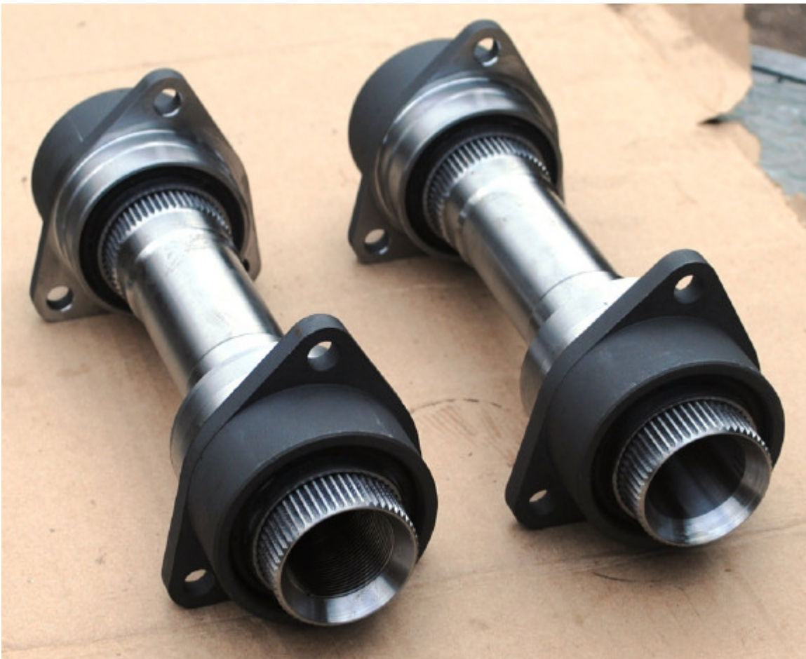
Fig 8 New silent blocs with their splined connecting pins
